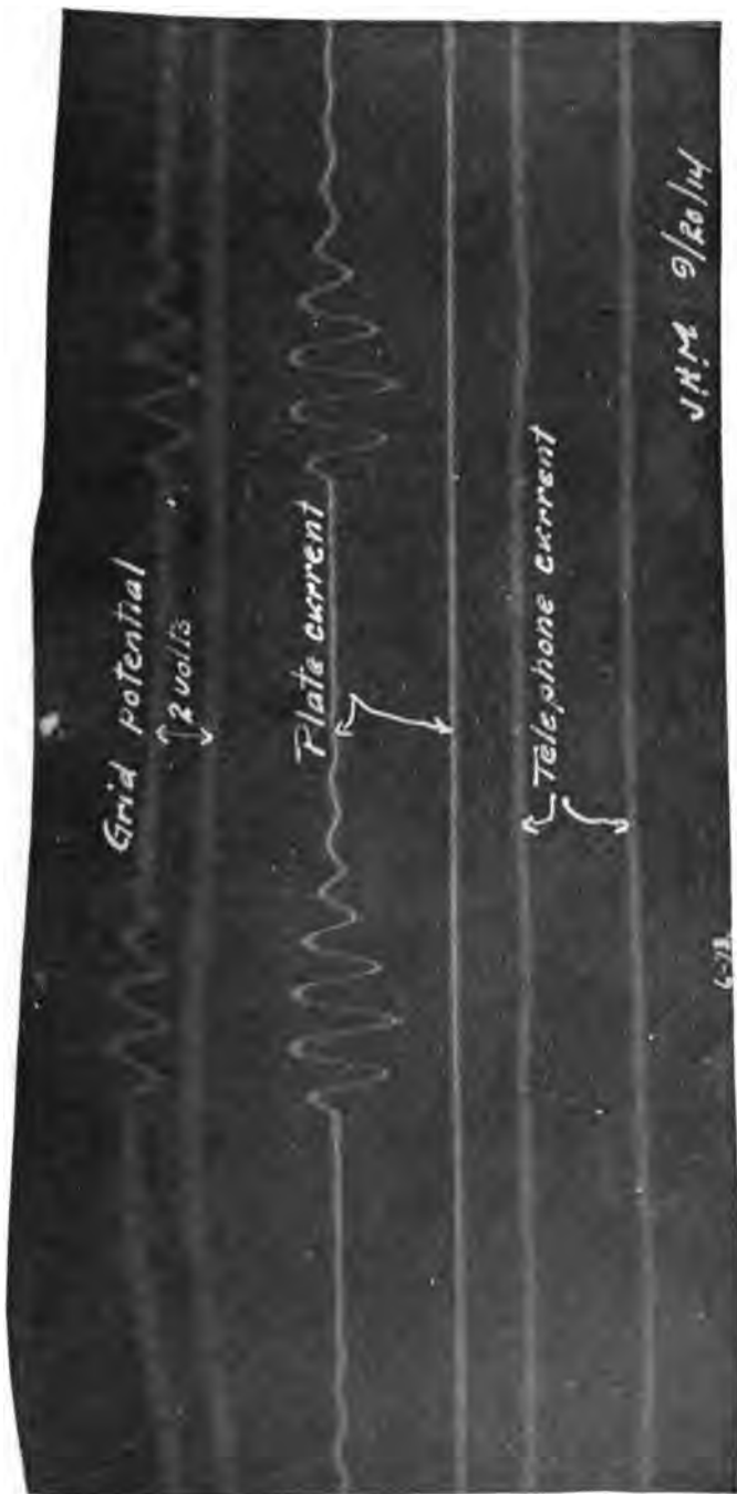
FIG. 73.—Rectifying action of tube adjusted for normal grid potential as at B, Fig. 72.
